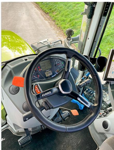
Our test team liked the grippy leather-clad steering wheel as well as the option of the parking brake position on the powershuttle. We didn't like the noticeable notches when shuttling back and forth between forwards and reverse.
