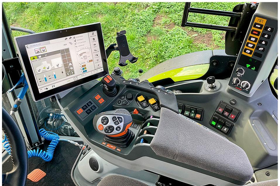
Good and sensible ergonomics – armrest, Cmotion stick and display. Elsewhere, the multitude of fixed switches feels outdated compared to other makes, though they're relatively simple to navigate.
