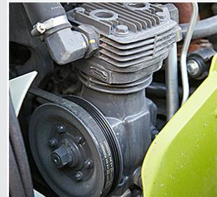
The compressor is too small, resulting in excessively long inflation times.
