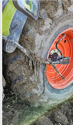
The externally routed tyre pressure hoses aren't optimal.
