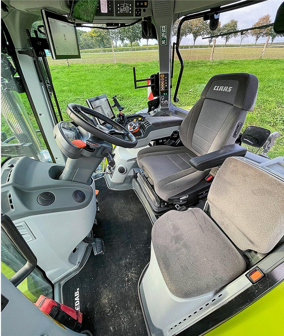
The cab is comfortable, but (too) short; taller operators will quickly identify this. At 74.8dB(A), the noise level measures louder than on other models, but the background noise isn't actually that bad.
