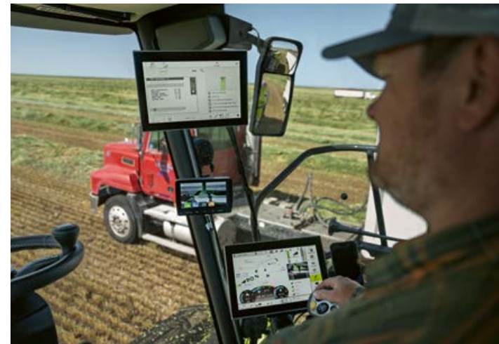
▲ CEMOS maintains the engine speed set by the operator and adjusts the engine output and ground speed in accordance with the volume harvested. CEMOS AUTO CROP FLOW provides overload protection. Page 44
