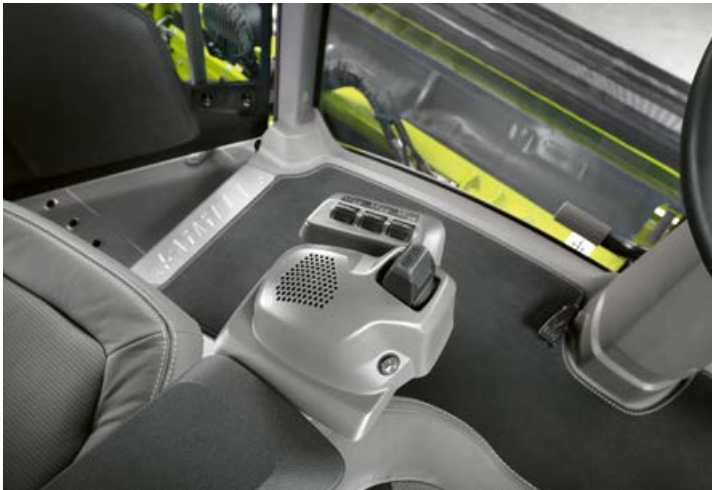
▲ Manoeuvring has never been more straightforward or effortless: the steering joystick and freely programmable function buttons are situated on the left-hand armrest. Page 42
