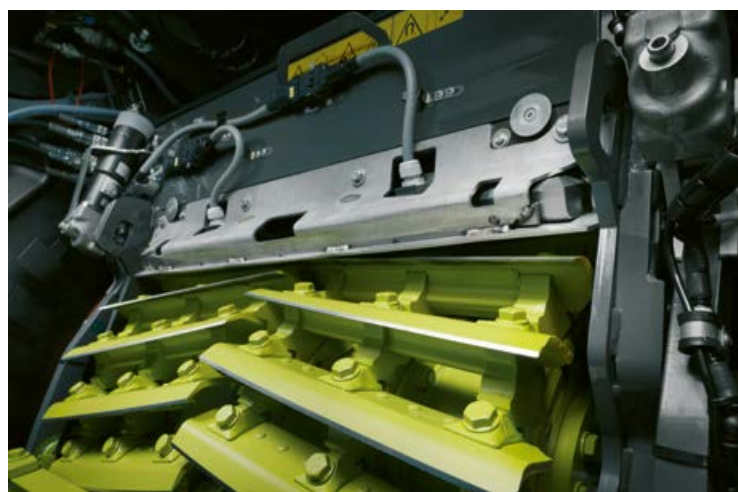
▲ NEW: CEMOS AUTO KNIFE CONDITION keeps the 910 mm wide V-FLEX chopping cylinder sharp at all times, thereby enabling precise chopping and an even crop flow. Page 26
