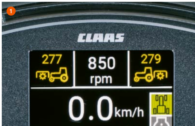
1 The digital speed indicator for the front and rear PTO means that you're always working at just the right speed
