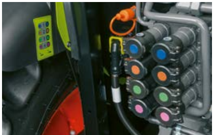
The rear connections are easy to identify thanks to colour-coding and adjacent stickers
