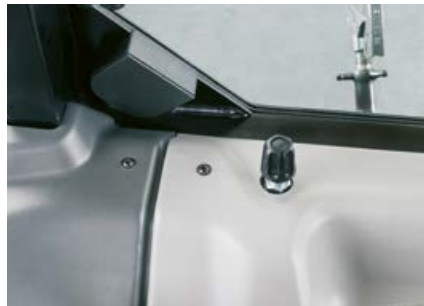
The maximum flow rate of mechanical spool valve 3 can be limited with just one hand from the comfort of the cab
