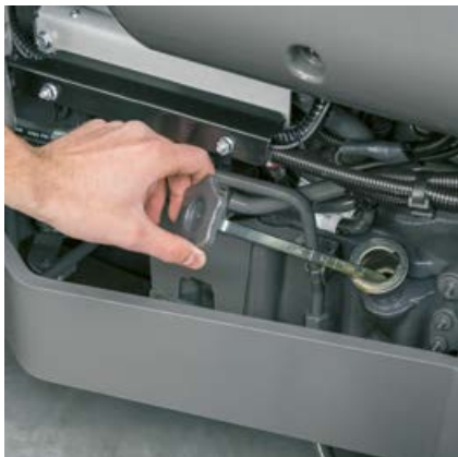
The oil level can be checked and topped up on the right-hand side of the AXOS 2 when the bonnet is closed
