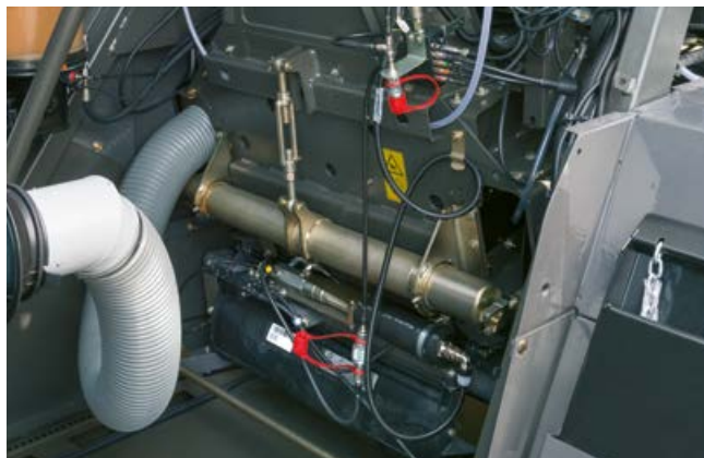
Mechanical adjustment of the crop accelerator clearance
