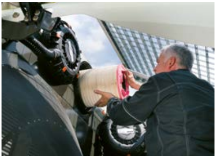
Air filter change without tools
