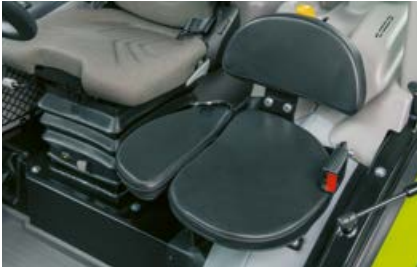
The wide passenger seat offers a comfortable ride, while the integrated retractable seat belt provides additional safety
