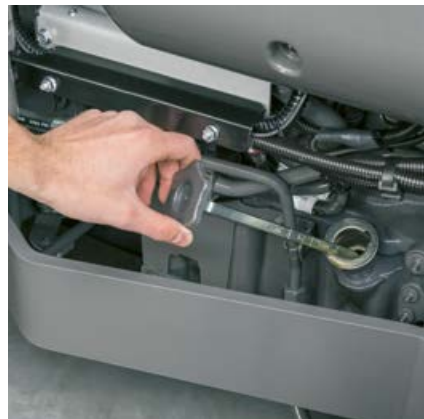
The oil level can be checked and topped up on the right-hand side of the ELIOS 3 when the bonnet is closed
