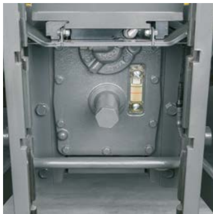
You can check the transmission and hydraulic oil level in a sight glass next to the rear PTO stub
