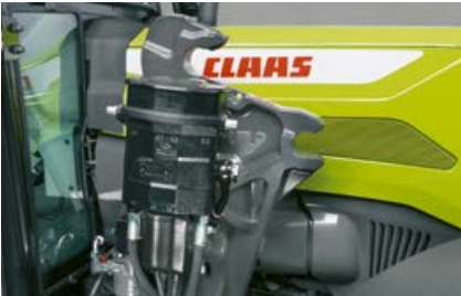
FITLOCK system for rapid attachment/removal and MACH quick-release coupler for electric and hydraulic connections
