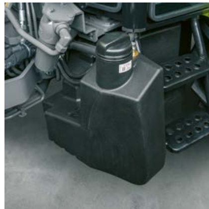
The 105 l diesel tank and the 10 l urea tank provide enough range for long working days
