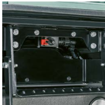
The battery isolating switch is conveniently located on the left access step
