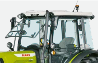
The front, rear and side windcreens can be opened for natural ventilation
