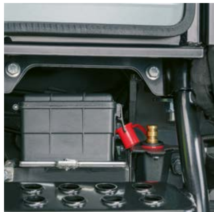
The ELIOS 3 incorporates a host of ingenious solutions designed to make your day-to-day work easier, such as the easily accessible battery terminals at the right hand side of the cab
