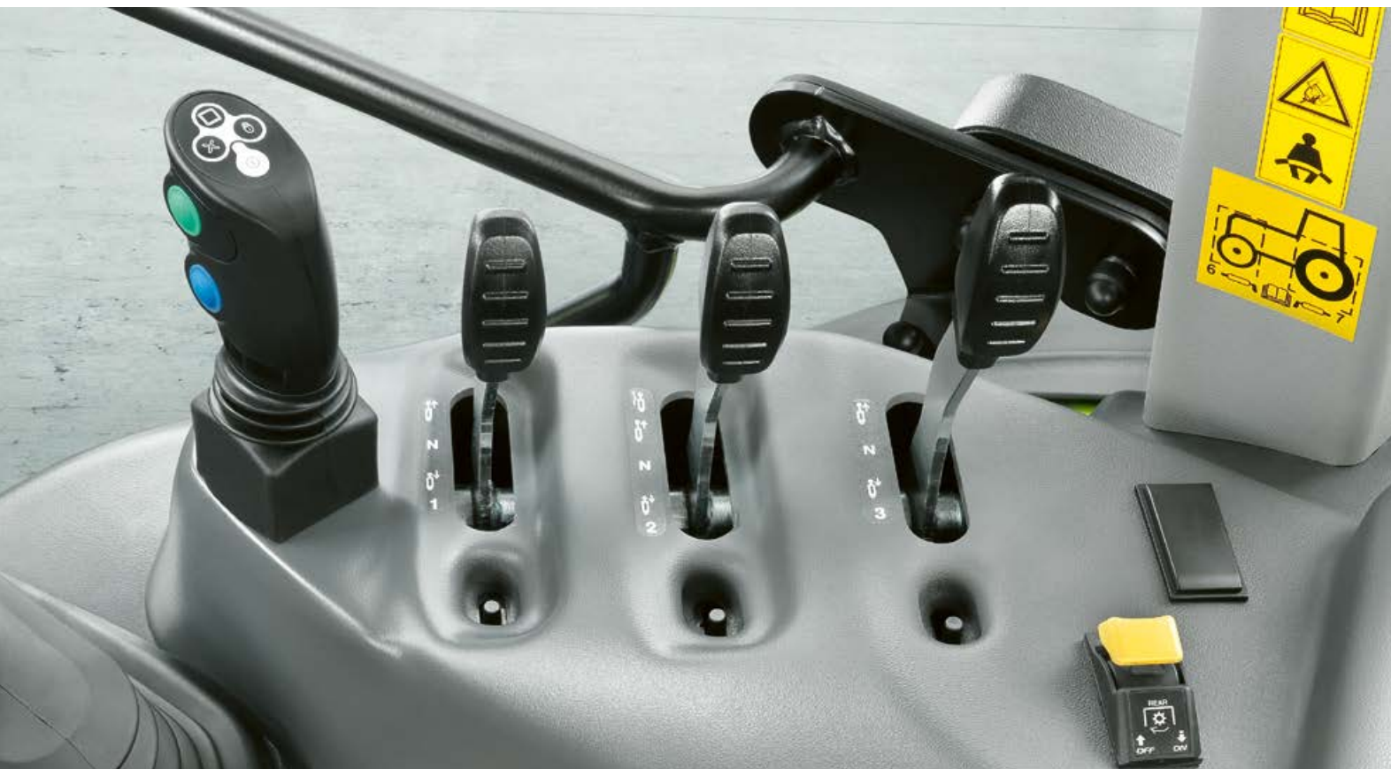
The maximum flow rate of mechanical spool valve 3 can be limited with just one hand from the comfort of the cab
