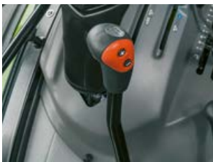
Choose a mechanical splitter on the right next to the steering wheel or the easy-to-use TWINSHIFT two-stage powershift which is operated from the gear-shift lever
