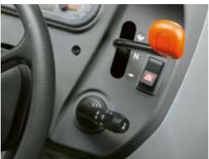
Choose a mechanical splitter on the right next to the steering wheel or the easy-to-use TWINSHIFT two-stage powershift which is operated from the gear-shift lever
