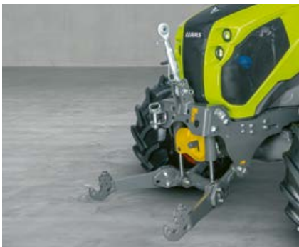
The optional front linkage with 3.2 t lift capacity and the front PTO extend the range of ELIOS 2 applications.
