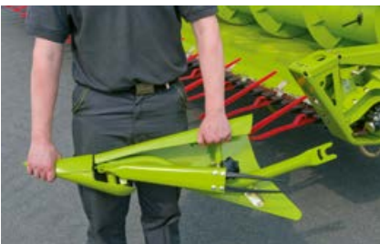
The crop dividers can be replaced quickly.
