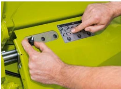
Setting the parking and cleaning position directly on the cutterbar
