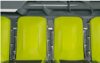
The picking plates are adjusted hydraulically.
