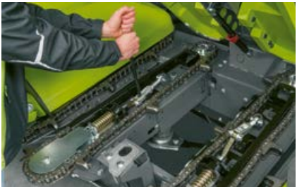
You can easily retension the conveyor chains.
