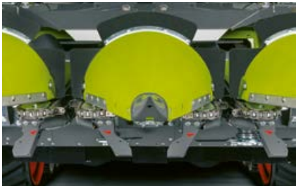
Rubber cob retainers make for a loss-free harvest.
