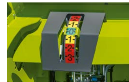
The current position of the knife bar is clearly visible from the cab.
