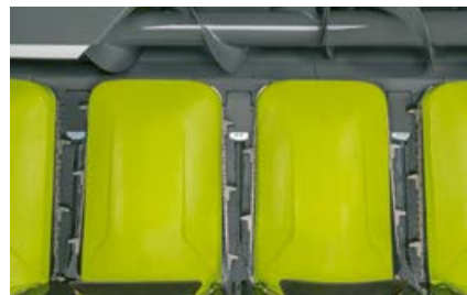
The picking plates are adjusted hydraulically.
