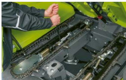
You can easily retension the conveyor chains.
