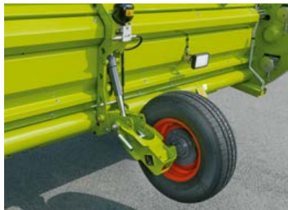
Two robust stabiliser wheels for improved ground adaptation
