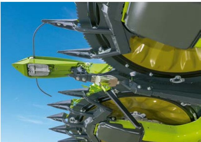
AUTO CONTOUR centre sensor, available for ORBIS 900.
