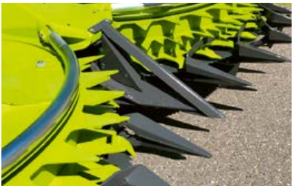
Efficient crop separation with narrow centre finger for crops with narrow stems.
