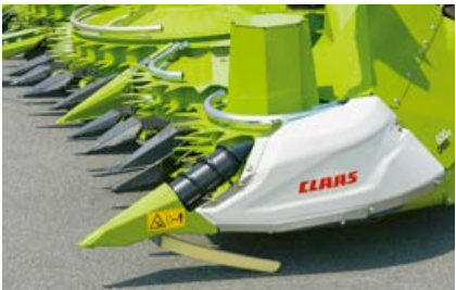
Hydraulically driven laid maize point.
