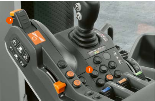
CIS+ operation 1 Change range 2 Activate cruise control
