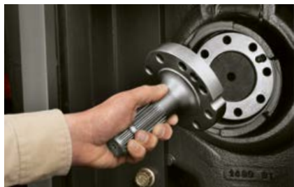
The PTO stub can be changed easily
