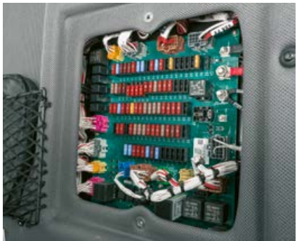
The on-board electronics is bundled for easy access.
