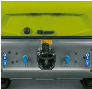
Two additional hydraulic quick-release couplers are provided at the rear.
