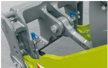
The machine is prepared for two more hydraulic connections.
