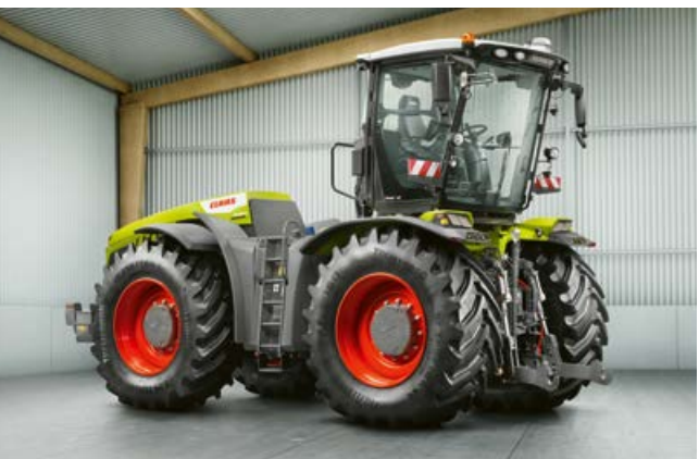
The TRAC VC has the most convenient reverse-drive system on the market. Its cab can be rotated through 180° in less than 30 seconds.
