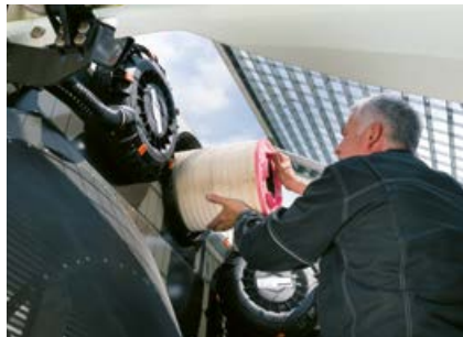
Air filter change without tools
