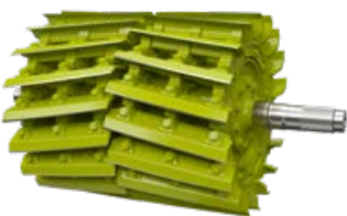
Full set of knives for short to medium lengths of cut.
