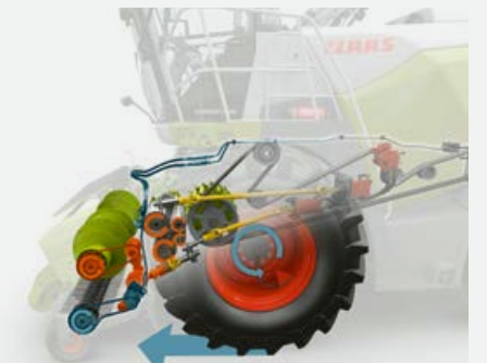
Variable front attachment drive
