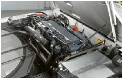
The TRION 760 and 750 models are powered by efficient six-cylinder MAN engines with up to 507 hp and a displacement of 12.4 l.
