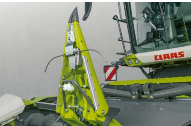
Two sensor bands each scan a row of maize.
