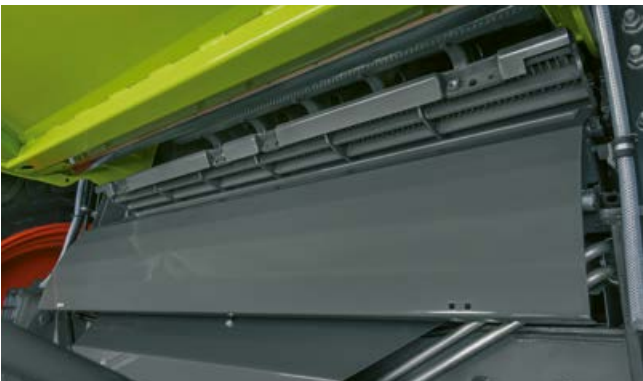
The concave segment can be pulled out easily through the stone trap.
