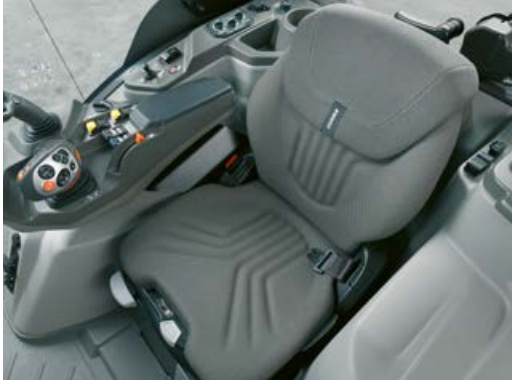
▼ The Premium seat with low-frequency air suspension, wide seat and backrest and integrated armrest take comfort to a new level in all NEXOS M, L and XL models.
