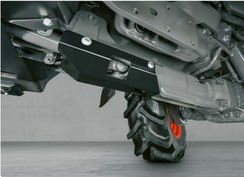
◀ The generous 80 mm spring travel cushions bumps with ease, and effectively evens out pitching movements during braking and acceleration.
