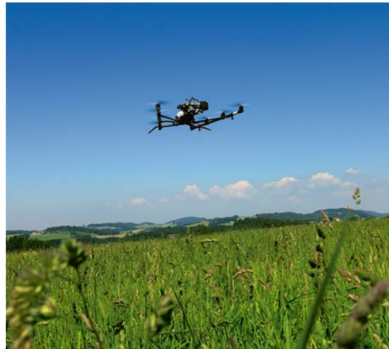
▲ Drones with infrared cameras scan the field. They can reliably detect fawns in long, thick grass from their heat signature
