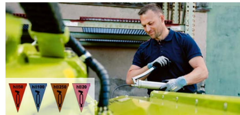
▲ Colour-coded lubrication stickers clearly indicate when each lubrication point has to be lubricated
