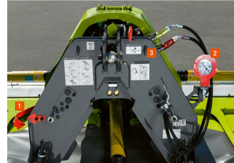
▼ All DISCO mowers have distinctive red markers to help you adjust them optimally: 1 Working height adjustment 2 ACTIVE FLOAT gauge 3 Kennfixx hydraulic hose indicator
