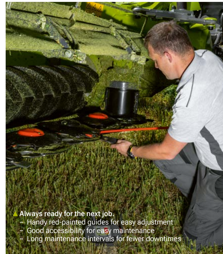
▼ All DISCO mowers have distinctive red markers to help you adjust them optimally: 1 Working height adjustment 2 ACTIVE FLOAT gauge 3 Kennfixx hydraulic hose indicator
