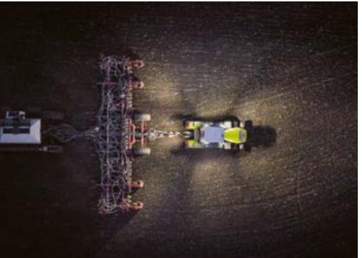
◀ The high-end lighting package with up to 22 LED headlights provides 53,400 lumen to illuminate your working area in a 360° radius.
