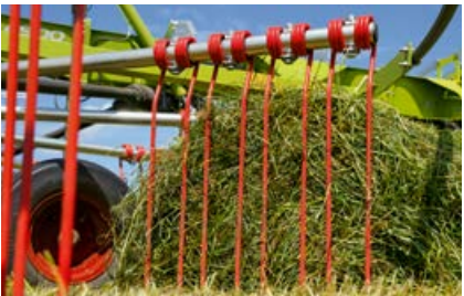
Silage tines for gentle forage handling
