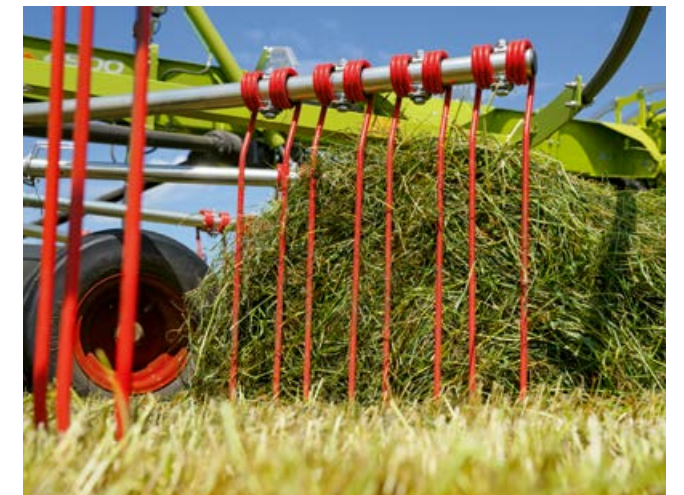
A tidy job – thanks to sturdy silage tines.
