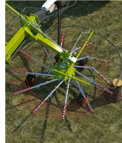
PROFIX tine arm attachment system.
