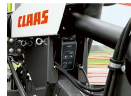
CEMIS 10 parking bracket for PLUS operation
