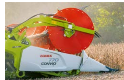
Spring-mounted crop dividers for harvesting crops growing close to the ground.
