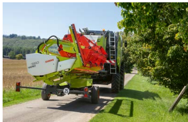
Even with rapeseed knives fitted, the VARIO cutterbars are compact enough for road travel on the transport trailer.
