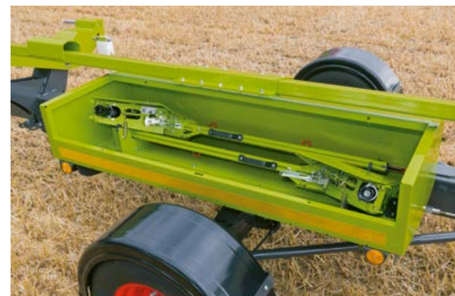
All transport trailers are equipped with a locking transport container that allows your rapeseed knives to be carried securely.
