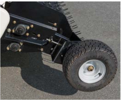
The working depth can be set by means of castor guide wheels.
