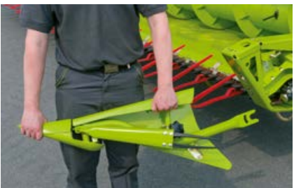
The crop dividers can be replaced quickly.
