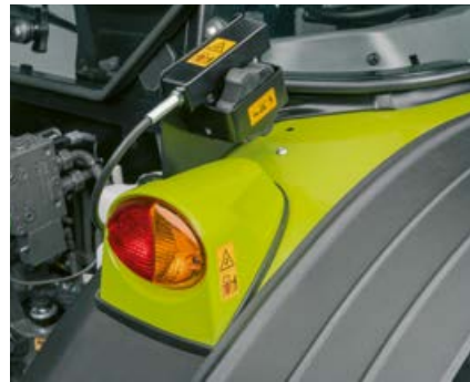
For implement attachment, the mechanical rear linkage can be operated externally at the rear of the tractor
