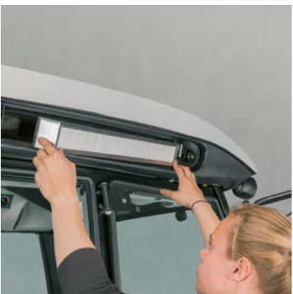
The cab air filter is easy to access from outside for cleaning and keeps the air in the cab fresh at all times
