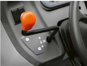
The reverser for mechanical reversing and the electronic REVERSHIFT are handily positioned to the left of the steering wheel
