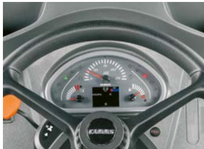
On the easy-to-read instrument panel you can see all the key information at a glance. The digital display shows additional operating parameters.
