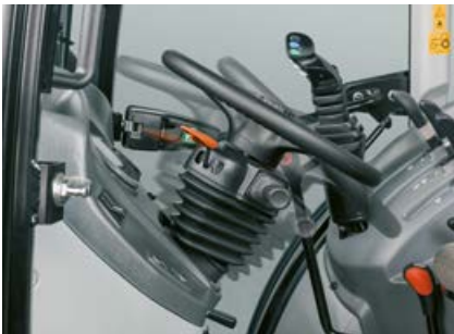
The steering column tilts and has telescopic height adjustment so it can be adapted to the driver's seating position
