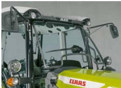
The front windscreen opens for natural ventilation
