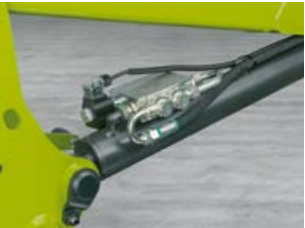
Thanks to electrical switching in the FL and FL C series, the safety valves can be combined with the SHOCK ELIMINATOR vibration damping system.
