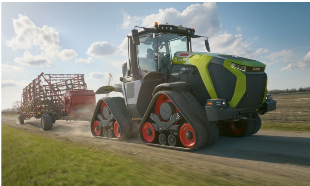
◀ The suspension design—from the shock-absorbing capabilities of the track assembly to the 4-point cab suspension and the cushioned premium seat—makes the XERION an exceptionally comfortable ride.
