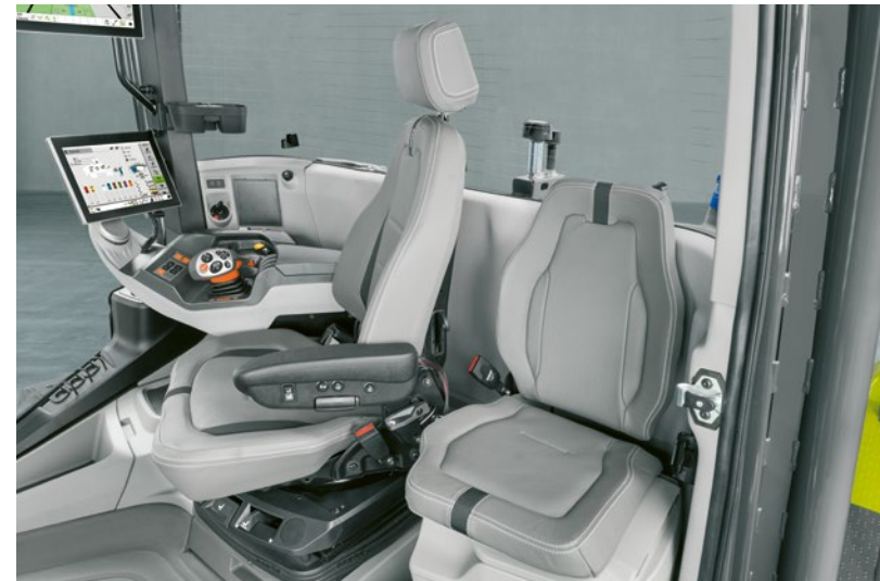
▲ Perfectly attuned to the needs of the operator, the XERION cab offers 21% more leg room, plenty of headroom for taller drivers and an abundance of storage space. Page 20
