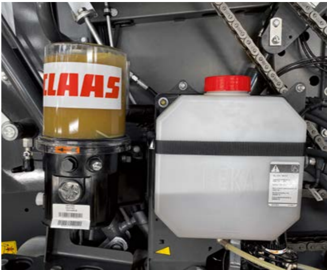
Central lubrication of the tailgate bearings.
