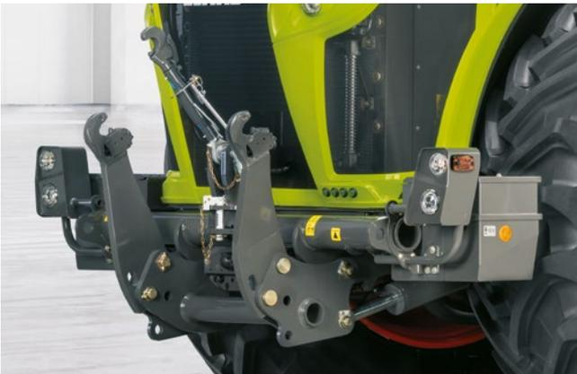
**8.9 tons lift capacity at the front.**
