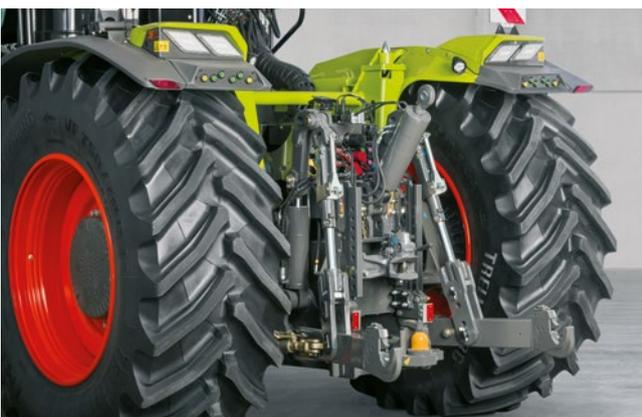
**11 tons lift capacity at the rear.**
