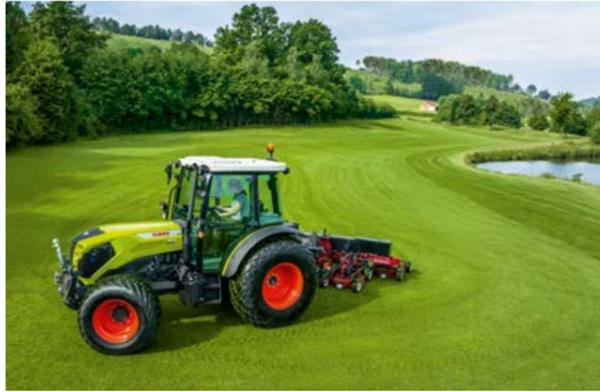
A low centre of gravity really comes into its own on difficult terrain such as sloping ground, giving the ELIOS tractors excellent stability. The maximum track width of 2,310 mm further reinforces this effect. Together with the balanced weight distribution, this ensures exceptional safety. And with a low unladen weight starting at 3.6 t, soil-friendly, fuel-efficient work is a given.
