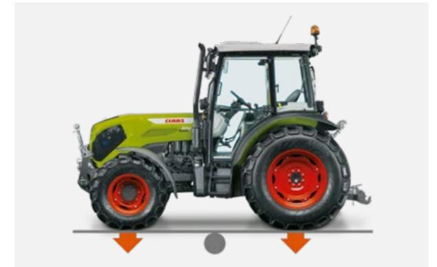
CLAAS supplies optional factory-fitted Trelleborg turf tyres (sizes: 600/55-26.5 rear and 00/55-22.5 front) to enable the ELIOS to be driven over sensitive grass cover or wet subsoil in parks and on sports fields without damaging the precious turf – all year round.
