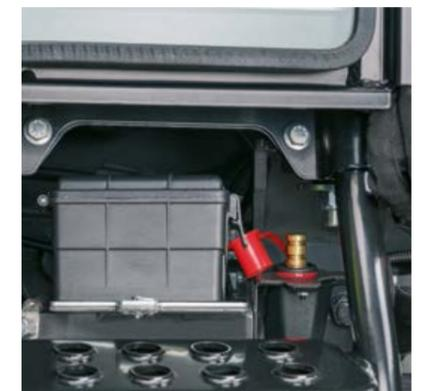
The ELIOS 300 incorporates a host of ingenious solutions designed to makes your day-to-day work easier, such as the easily accessible battery terminals at the right hand side of the cab
