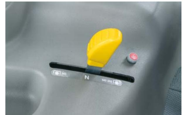
The electrohydraulic PTO engagement controls the start-up smoothly to suit the attached implement and protects the mechanical components
