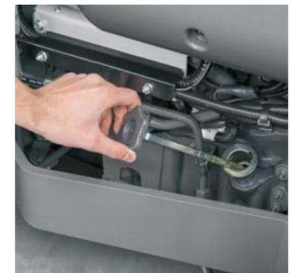
The oil level can be checked and topped up on the right-hand side of the ELIOS 300 when the bonnet is closed
