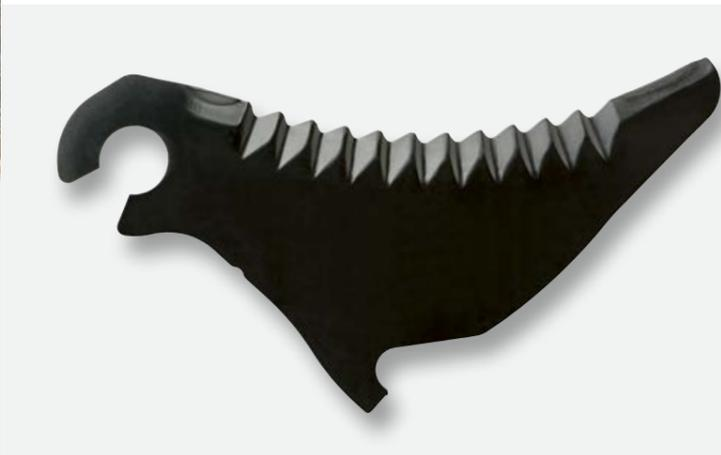
Regarding the cutting quality, the solid heavy-duty cutting rotor in the ROLLANT is designed for ultimate performance. It is made of double-hardened boron steel with helical double tines. Individual blade protection prevents damage to the knives, increases their service life and ensures consistent cutting quality. The knives are also available with tungsten carbide coating.
