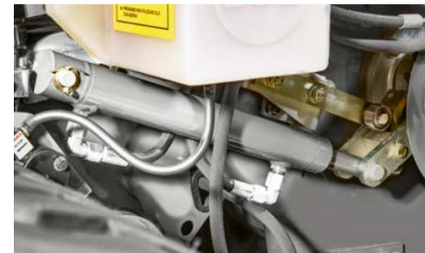
Blockages in the intake can be cleared quickly and easily by reversing the rotor mechanically using the rotor lever. The optionally available hydraulic rotor unblocking unit can be activated from the cab and allows the baler to be driven right up to its performance limits without any problems.
