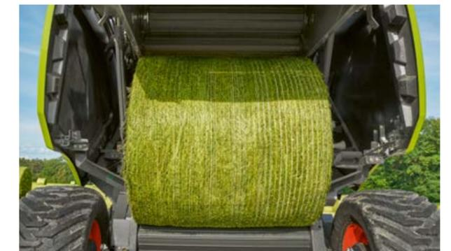
The CLAAS ROLLANT is the world's top-selling fixed chamber baler. Its proven, robust fixed-chamber concept is continually being enhanced by CLAAS engineers. The ROLLANT 540 features the latest generation of rollers with 15 reinforced rollers, 50-mm drive stubs and extra-robust ball bearings for perfectly formed silage bales and optimum crop flow.
