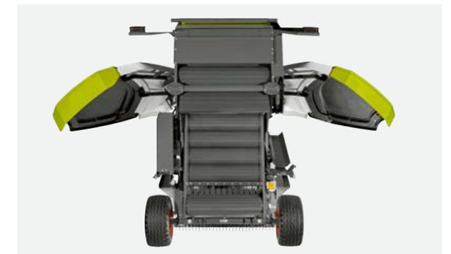
The 17 HD rollers, with a significantly thicker casing, process the crop into firm 1.22 x 1.50-m bales with excellent shape retention – with net wrapping or twine tying as desired.
