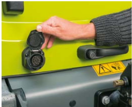
13-pin rear socket for use with a trailer
