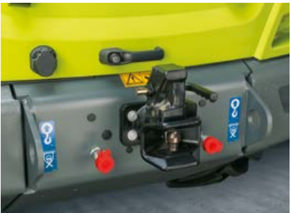
TORION 956 SINUS optionally with a pressure-free hydraulic return at the rear
