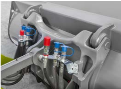
All connections are easily accessible and well-protected on the implement carrier (956)
