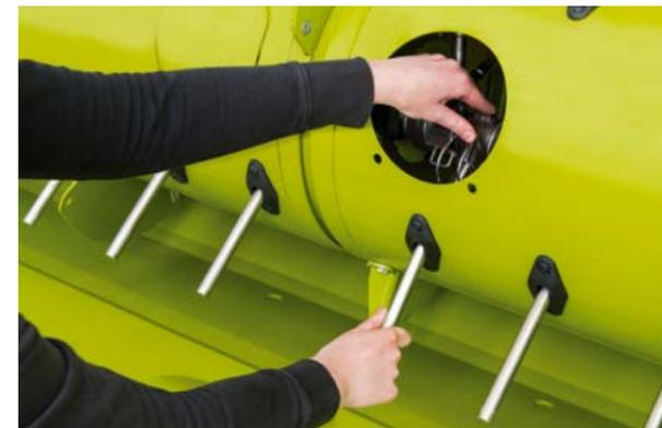
**Intake auger fingers replaceable without tools.**
