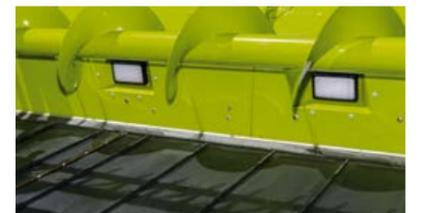
Powerful work lights illuminate the cutterbar and trough perfectly
