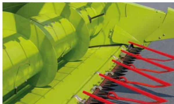
Cutterbar table retracted – grain (-100 mm)
