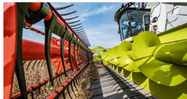
Cam-track-controlled reel with flip-over concept
