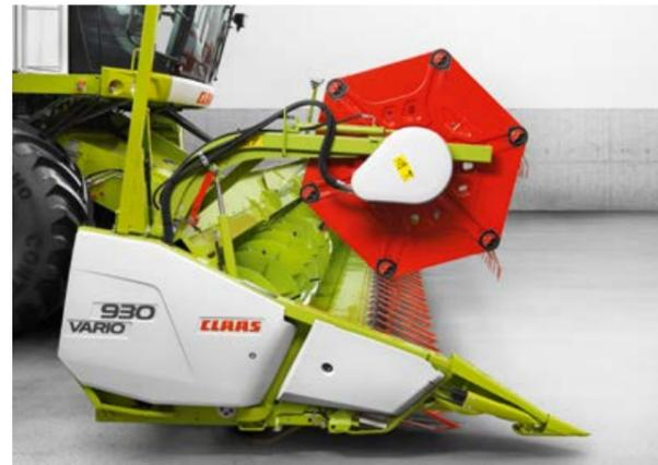
Cutterbar table retracted – grain (-100 mm)
