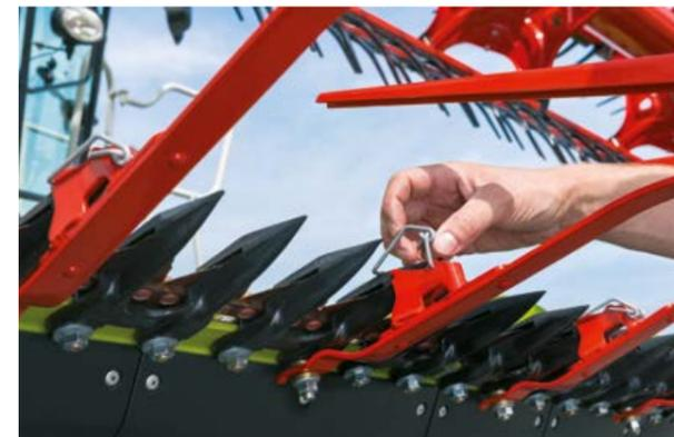
**Crop lifters can be replaced quickly.**
