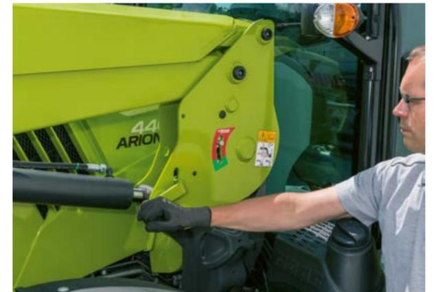
From your driving position in the cab, a glance at the lock indicator is all it takes to check that the lift arms are properly engaged. Detaching the loader is just as quick and easy.
