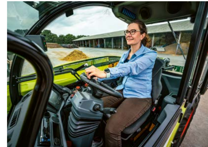
▲ Informative terminal. Key parameters and the current operating status of the machine and units are always in view. The sub-menus are easy to understand. A 7" colour display is also available as an option.
