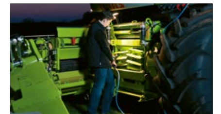
QUICK ACCESS lets you inspect the chopping unit in a matter of minutes.
