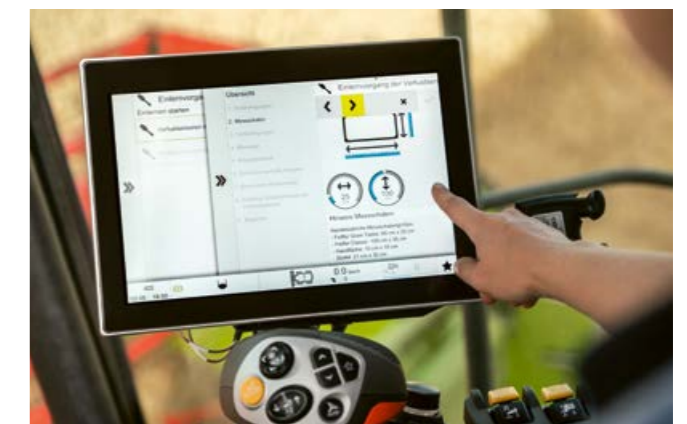
The dimensions of the loss control pan being used are entered in CEBIS
