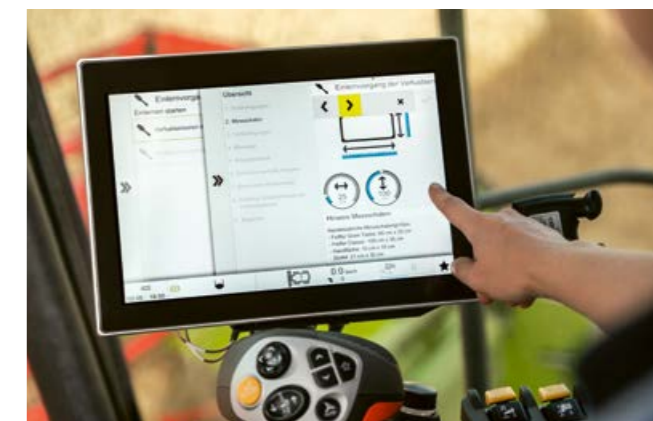
The dimensions of the loss control pan being used are entered in CEBIS
