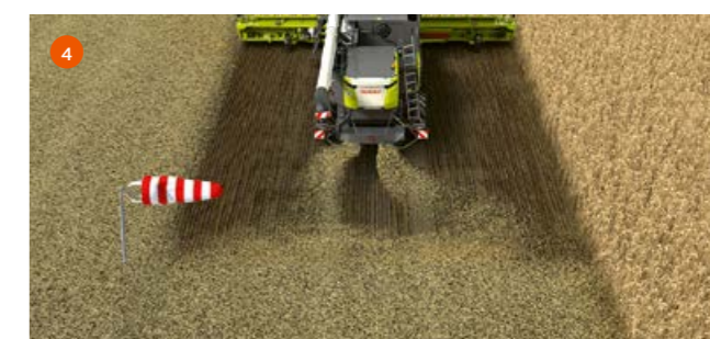
3 Sensors at the rear of the machine detect the intensity of the crosswind.
