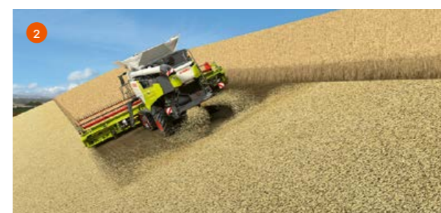
1 If the machine is operating on a slope, the discharge direction is adjusted automatically.
