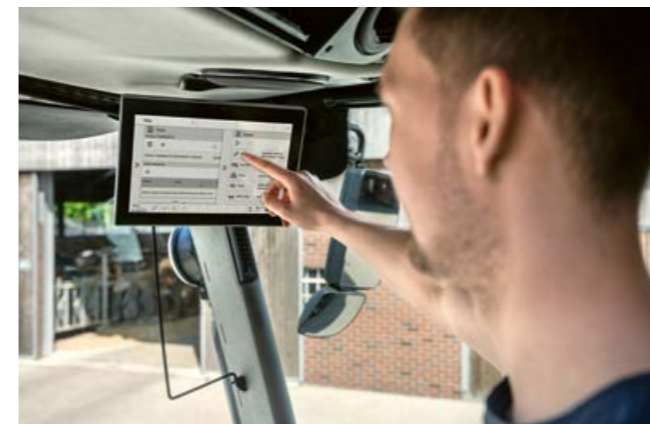
With CEMIS 1200, all jobs can be created and managed directly on the machine.
