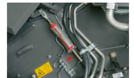
All lubrication points are combined and clearly indicated in grease anchor blocks.
