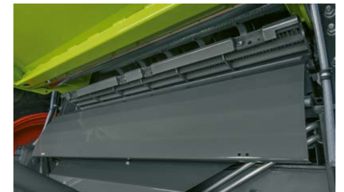
The concave segment can be pulled out easily through the stone trap.
