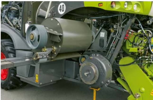
Easy removal and installation of the accelerator
