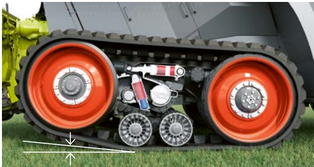
66% contact area: the track roller is raised when negotiating curves.
