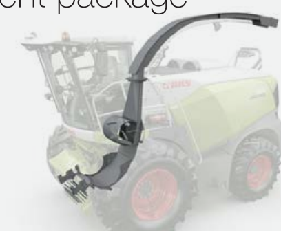
PREMIUM LINE crop flow with shear bar
