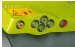
External controls for the rear linkage, PTO and one freely selectable spool valve (CEBIS only)
