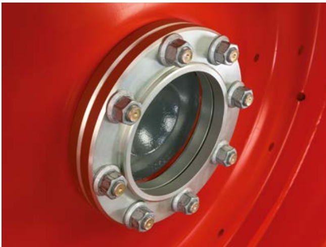
Wheel spacers to adjust the track and quick-release axle available as an option
