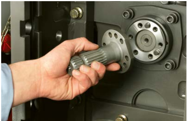
The PTO stub is easy to change
