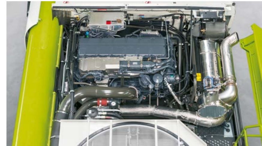
MAN D42 with 581 kW / 790 hp for LEXION 8900 / 8800.
