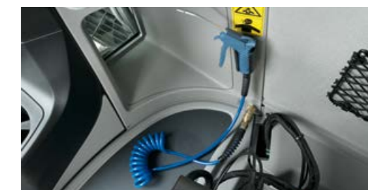
For quick cleaning on the go – the air pressure gun in the cab
