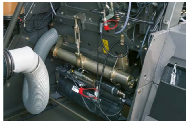
Mechanical adjustment of the crop accelerator clearance
