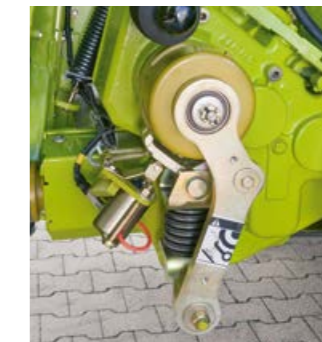
Metal detector power interrupt clutch
