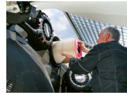
Air filter change without tools
