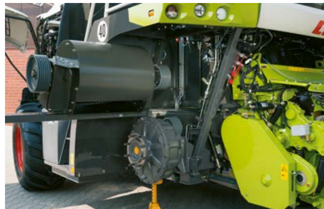
Easy removal and installation of the accelerator
