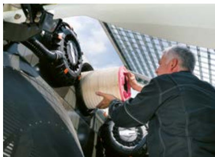
Air filter change without tools
