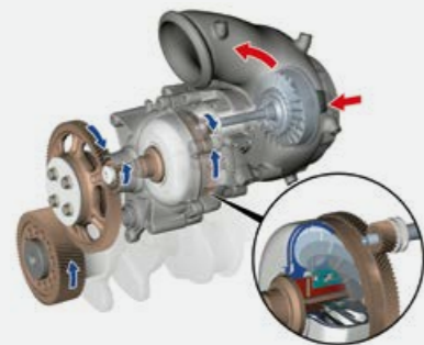
Turbo-compound technology for OM 473 LA
