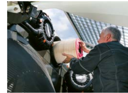
Air filter change without tools
