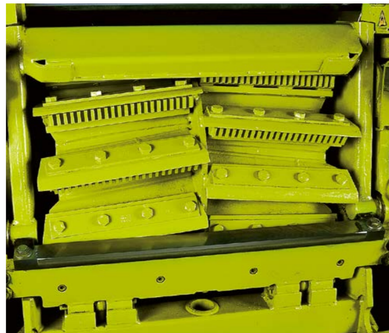
Micro-profile rasp bars under the knives for additional crop processing
