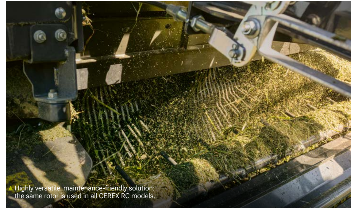
▲ The PRO lowerable floor actively adjusts to the crop flow.
