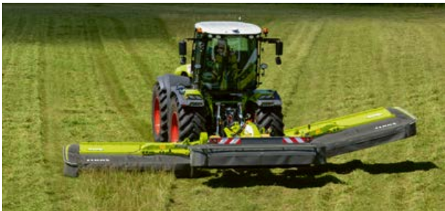
Individual mower unit lift at the headland
