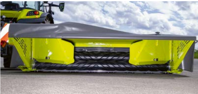
Two additional telescopic swathing plates are optionally available for roller conditioners.
