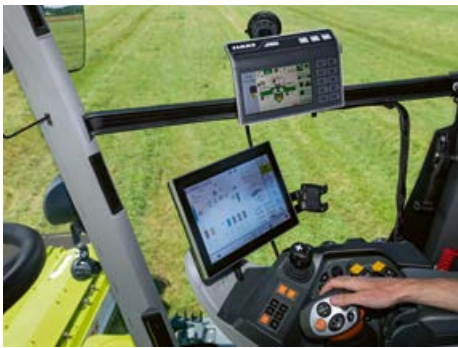
Comfortable operation, for example via a range of ISOBUS terminals and the ISOBUS function keys on the control lever
