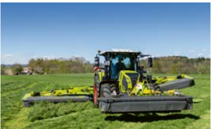
The compact hitch gives the mower generous ground clearance at headland
