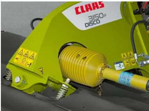
Intelligent transverse oscillation with angled pivot point ensures a clean cut and protects the sward
