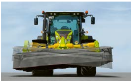
The freely floating suspension compensates for uneven ground across the direction of travel
