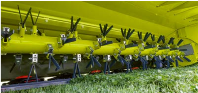
The wear-resistant Hardox conditioner hood ensures a long service life even under extreme conditions.
