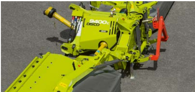
Hydraulic non-stop collision protection – in the event of a collision, the mower swings up and over the obstacle, and resets itself automatically
