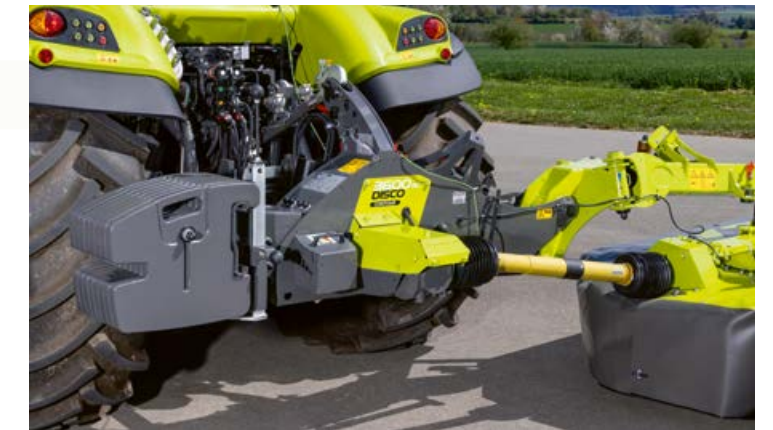
▼ Optional counterweights provide more stability, higher ride comfort and safe deployment on hilly ground.
