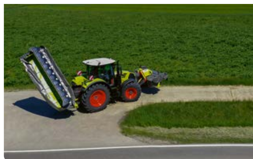
▼ Even the biggest DISCO folds up small: compact transport position despite 4.20 m working width
