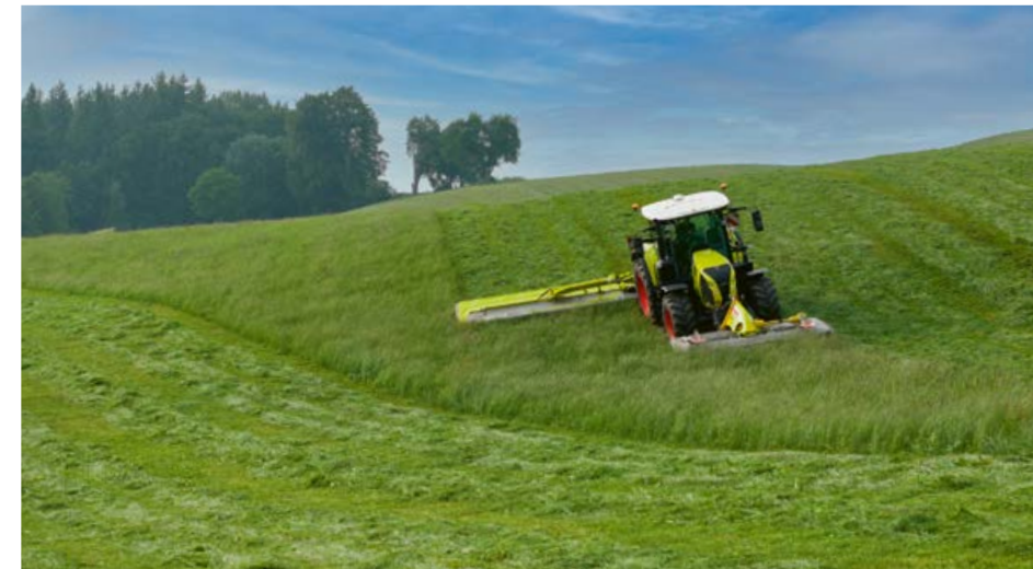
▼ Ground-contour following even on slopes. The mower units of the CONTOUR series pivot freely and follow the ground contours precisely.
