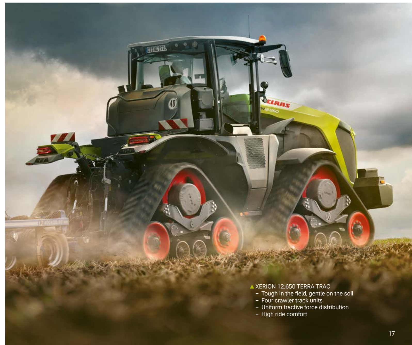
◀ Two belt widths (914 mm or 762 mm) guarantee maximum ground protection. With the narrower track belts, the overall width of the XERION is less than 3 m.
