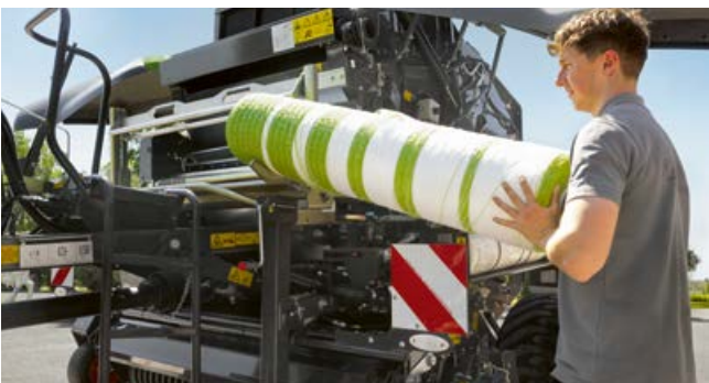
The new net wrapping system in the VARIANT 500 series is positioned 25 cm lower to allow easy cleaning of the net roll under the net brake.
